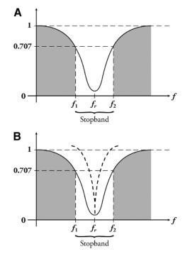
**FIGURE 6.** A, a typical-appearing stop band. B, a stop band suggesting that the "notch" has become much more narrow, thereby making it more difficult to locate.
